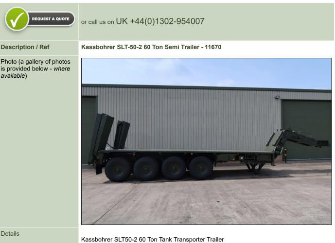
Length (overall) 13.1m Width 3.2m Track 2.65m Height (overall) 3.15m Fifth wheel height 1.55m Load area Length 8m Height from ground 1.3m Ground clearence 0.30m Weight 16,600kg
